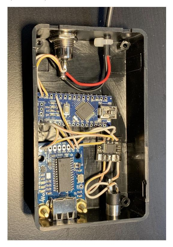
Here is a photo of the completed converter box for USB use:
