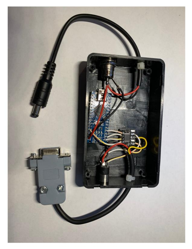
Detail on the wiring between the RS232 interface (right) and the Arduino (left). The red and black wires to the Arduino are for power, the various wires to the bottom right are for the DB-9 and RH96 serial data.
